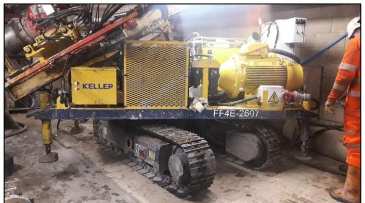
The Keller electric FF4 rig that will be used at 90 Long Acre for the piling.
